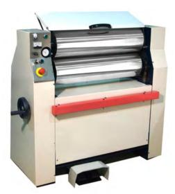
For applications where personnel operate the machine, a Guard in front of the Gap between the mixing rolls fully guards the entrance. When this guard is part of the machine, compressed air operates the guard, an essential requirement.
